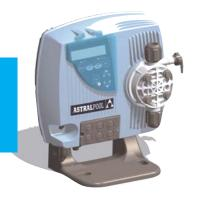
Systems produced according to EC standards. IP65 protection. 90-65 VAC 50/65 Hz electrical power supply. Materials in contact with the chemical product are made of polypropylene, Viton, Teflon and PVC (other materials possible upon request). Anti-acid plastic container. Moisture-resistant membrane buttons. Built-in relief valve. No lubrication necessary, minimum maintenance.
